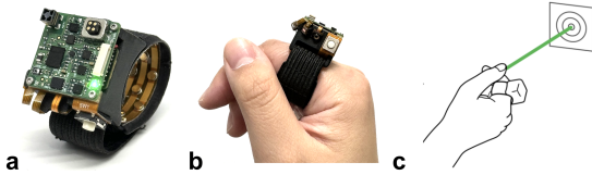
Figure 4: (a) Ring hardware (ElectroRing [29]) with a 9-axis IMU and embedded electrodes; (b) “thumb tap” gesture for selection; (c) the ring pointing posture used during interaction and calibration.
